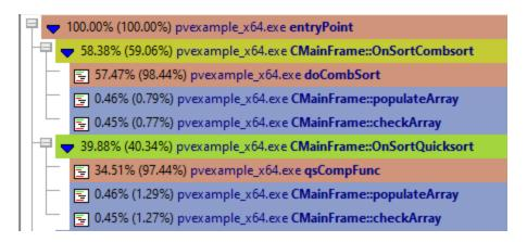
• Total % > colouring is based on function time relative to the total execution time
